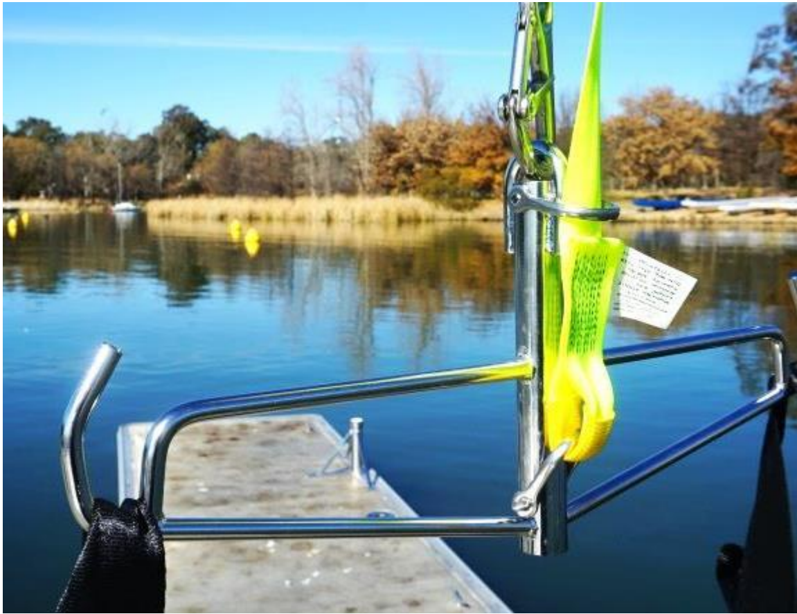
Spreader Bar with Fall Arrester/safety line and sling attached
